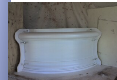
3. (Above) Finished face of plaster model ready to receive slurry of mold-forming material to create "negative" mold.
