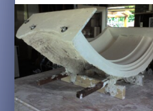
5. (Above) Same mold with armature turned flat. Ready to receive curved plywood inside radius closure and final "positive" cement pour.
