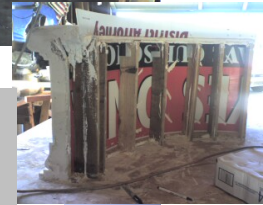
2. Back side of screeded plaster model of quarter segment (right)
